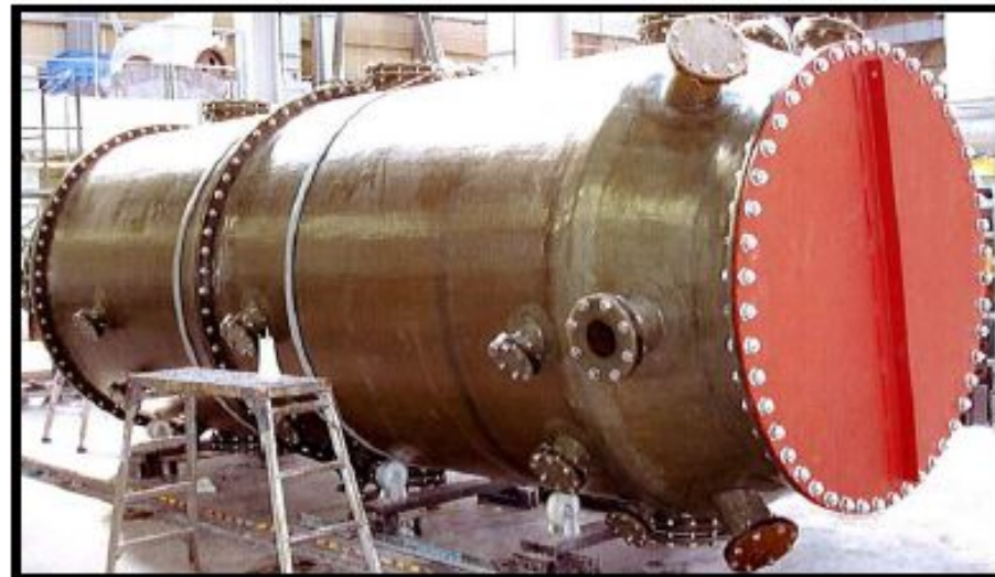
Φ1,800 × 5,500mmH Gas Volume(wet) : 10,000 ~ 40,000 m 3 N/h Dust Content : In put 0.15 ~ 0.20 → Output 0.003 ~ 0.004g/m 3 N
