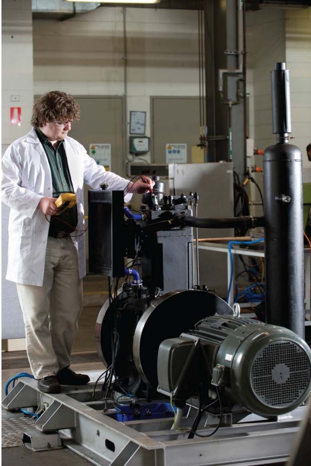
8 kw diesel engine test
